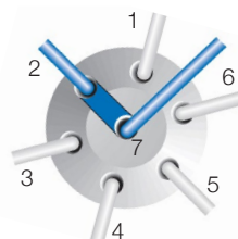
Flow path of Six-Position, Seven-Port Selector Valve
